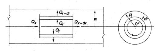
The energy equation for a fully developed flow in a tube is reduced to
