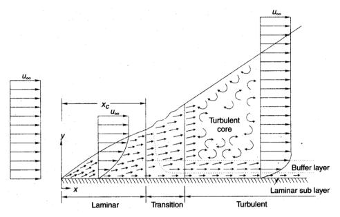
Depending upon the flow field and fluid properties, at some **critical distance** from the leading edge small disturbances in the flow begin to get amplified, a **transition** process takes place and the flow becomes **turbulent**.
