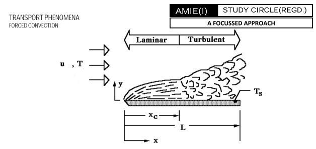
Defining the boundary layer thickness,  $\delta$ , as the value of y for which  $u/u_{\infty} = 0.99$ ,
