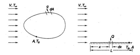
Local heat flux, 'q' for an arbitrarily shaped surface of area A at temperature  $T_S$ , over which flows a fluid of velocity V and of temperature  $T_{\infty}$  is given by
