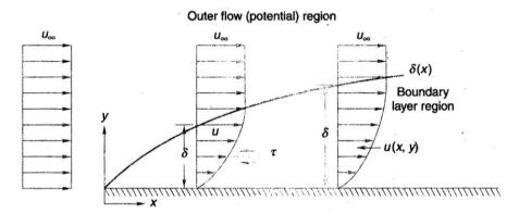
The velocity here in front of the **leading edge** of the plate is **uniform**. Due to the no slip condition to be satisfied at the surface of the plate, the velocity of the fluid is reduced to zero relative to the surface. This results in the retardation of the fluid particles in the adjoining fluid layers until at a distance  $y = \delta$  from the surface (called **boundary layer thickness**) this effect becomes negligible.
